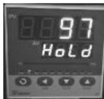
In Hold state, press the
